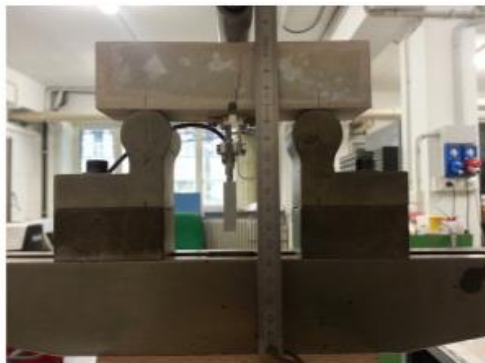
Figure 6. Specimen under load during the pre-loading stage with maximum CMOD of approximately 800\ \mu\text{m} .
