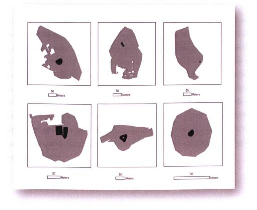
Figure 6; Typical Cost Weighted distance buffers (grey) at 250m effective distance from pond polygons (black). Note areas internal to buffers considered inaccessible, i.e. "beyond" the buffer distance due to land cover characteristics (white in grey).
