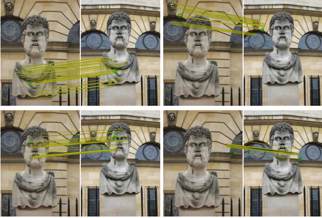
Figure 7: Several pairs of matching feature maps and the corresponding inliers after rectified feature selection, following the example of Figures 4 and 5. Inliers are less than in Figure 5, but still enough to match the images, especially since inliers are summed over all feature maps. Note that these are not the only pairs of maps with inliers for the images shown.
