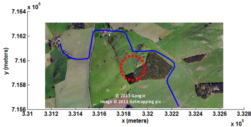
Figure 3: The trajectories of the simulated UAV (red stars) and vehicle (blue line) movements. The satellite image is taken from Google Earth and geo-referenced.
