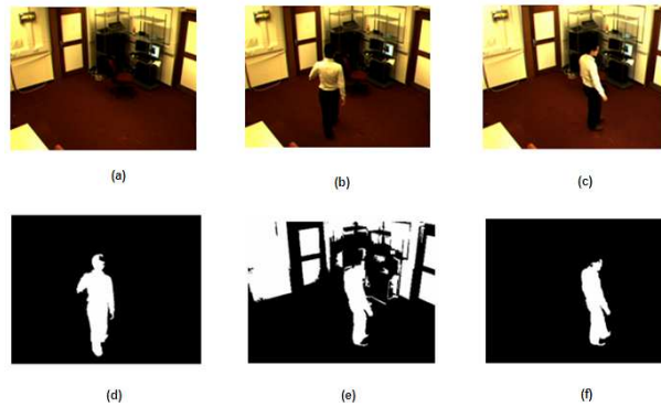
Fig. 5. Background subtraction results under sudden change of the light condition. (a) Original background image. (b) Image with foreground subject before the illumination change. (c) Image with foreground subject after the illumination change. (d) Background subtraction result under initial background model. (e) Background subtraction result under sudden illumination change. (f) Background subtraction result under retrained background model.
