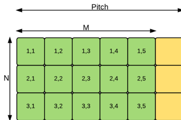
Figure 6.2: 2D matrix allocation. When allocating device memory via the cudaMallocPitch function call, rows are padded (yellow blocks) to guarantee that the beginning of each row begins on a 128 memory boundary.
