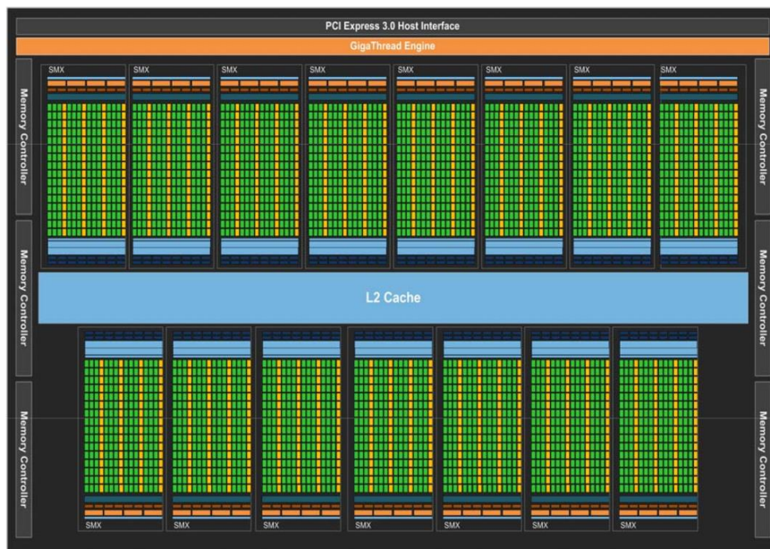
Figure 5.1: Kepler GK110 Full chip block diagram (Source: NVIDIA, 2012, p6)
