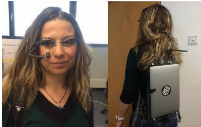
Figure 3.4. Illustration of the Positive Science mobile eye tracker system. The left image shows the head-gear, with the infrared diode and eye camera mounted below the participants' right eye. The image on the right shows the laptop attached to the backpack that serves to collect the eye movements and for controlling the system.
