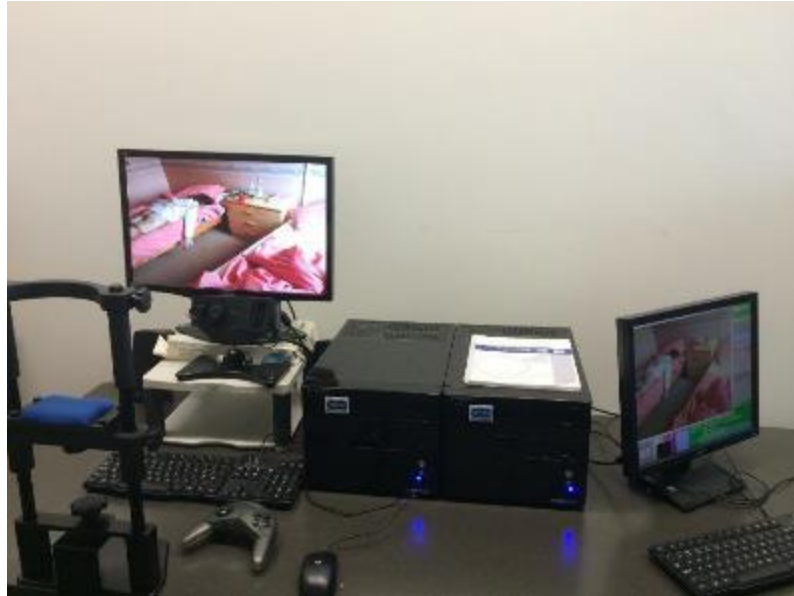
Figure 3.3. An Image of an Eyelink 1000 desk mounted eye tracking system with the chin rest. On the left is where the observer sits, with their head in the chin and head rest, looking at the computer screen, showing the stimulus (a crime scene here). In the middle are the two computers, one used for stimulus presentation (left computer), and the other for recording and parsing the eye movement data (right computer). The experimenter sits on the right and has a view of the image shown with a cursor superimposed indicating the estimated viewing direction of the observer. A view of the image of the eye is provided as well, providing a monitor to determine whether settings are still optimal for accurate eye tracking data.
