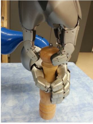
Fig. 5. The grasp used during the pepper mill grasping and turning experiment.
