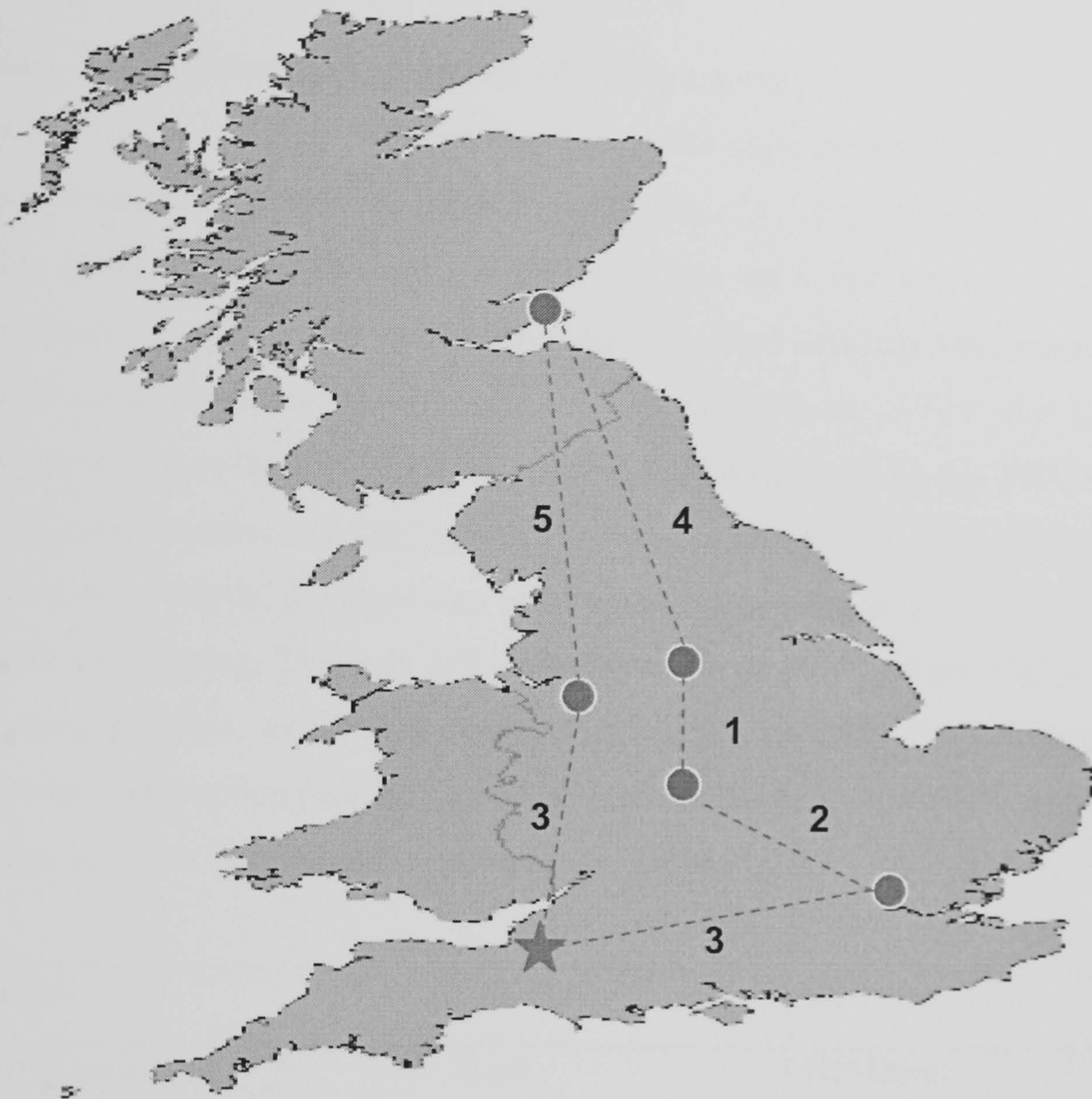
Fig. 4.1. An example of a travelling salesman tour, where the circles represent the cities the travelling salesman has to visit and the dashed lines are the trip from one city to another and on the dashed lines there is a set of weights corresponding to the distance covered. The start and the end city are marked by a star.
