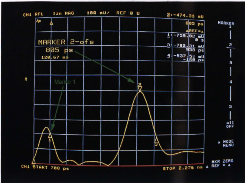
Figure 4-9 A typical TDR trace on the HP 8752C Network Analyser.
