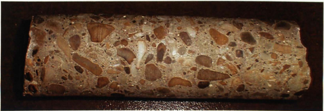
Figure 3-6 Core drill sample of a typical concrete showing the range of aggregate sizes used.
