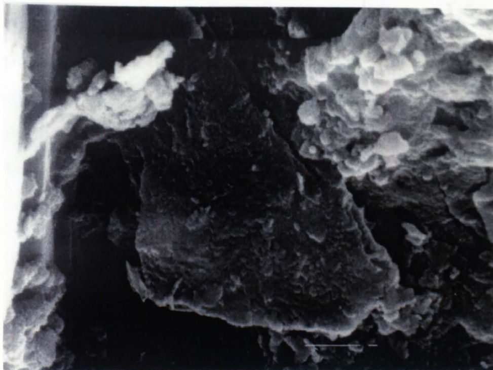
Figure 3-5 SEM of cement paste near a crack.
