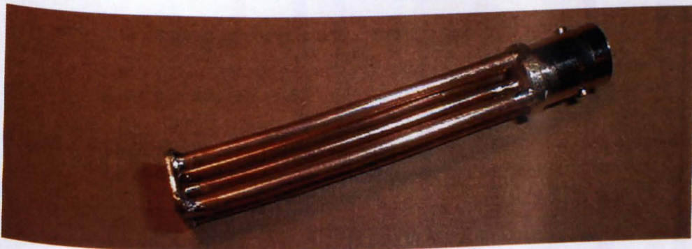
Figure 4-6 The cage-coaxial transmission line before being cast into cement.
