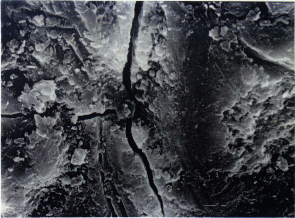
Figure 3-4 Micro-crack width about 500 nm at the widest point in cement paste.
