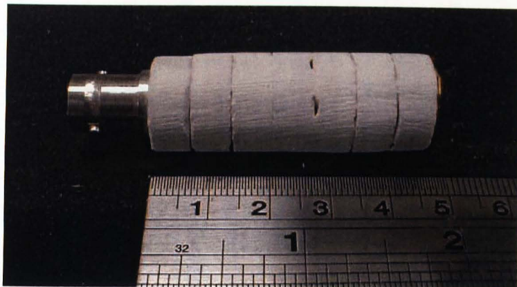
Figure 6-5 Photograph of transmission line with ceramic wafers
