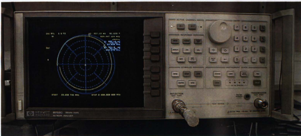
Figure 4-8 The HP 8752C Network Analyzer. The display shows a polar diagram for phase measurements.
