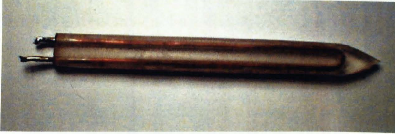
Figure 6-1 Two-wire transmission line embedded in acrylic.
