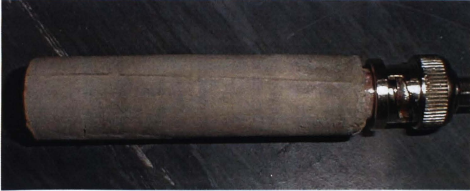
Figure 4-7 The transmission line after being cast in cement or mortar. Dimensions are: length = 60 mm, diameter = 15 mm
