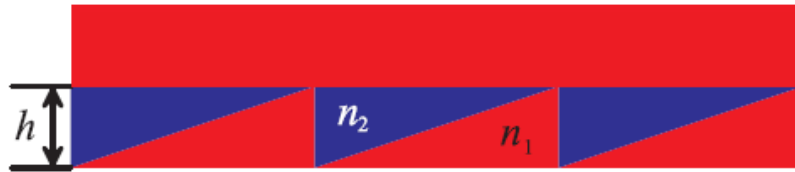
Figure 3.21: Diagram of the cement concept of the multilayer HAD. n_1 is the refractive index of the material and n_2 the refractive index of the cement material
