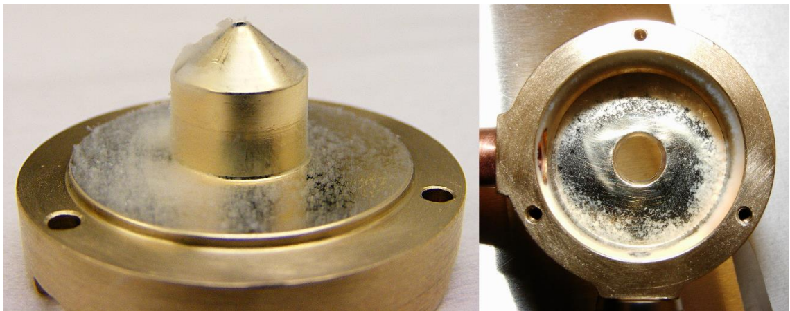
Figure 118: Photographs of the interior of the polished extraction head after the third long cutting trial. The top piece is on the left, lower piece on the right.
