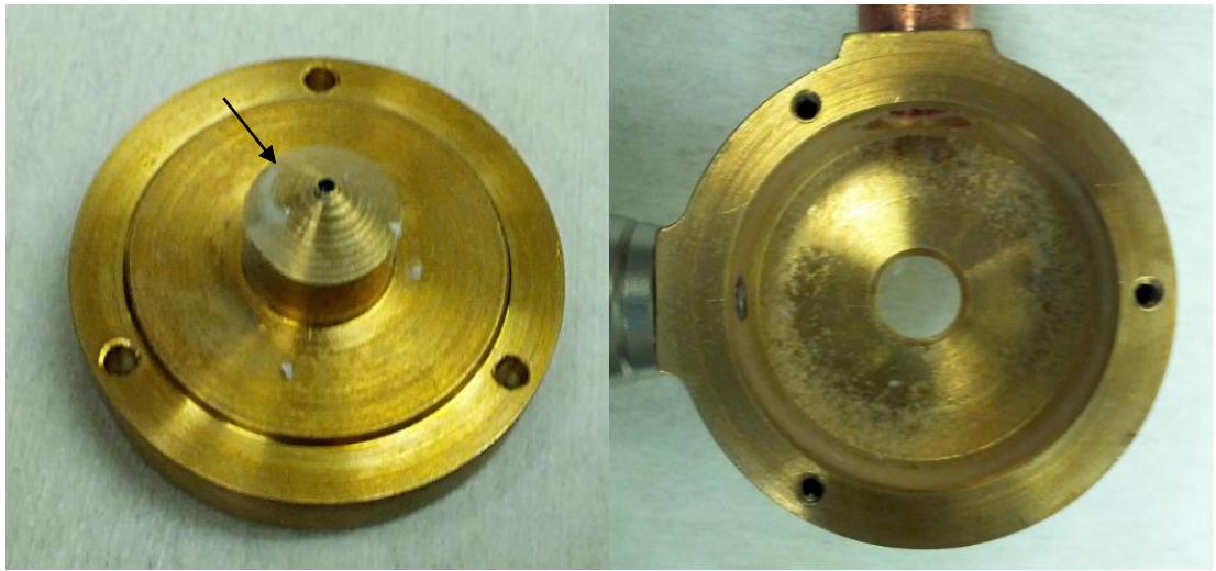
Figure 111: Photographs of the interior of the extraction head after the long cutting trial. The top piece of the assembly is on the left and the lower piece of the assembly is on the right. The black arrow indicates where some of the veneer-type deposit was removed.
