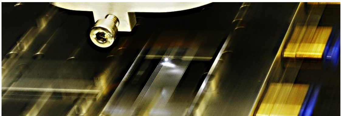
Figure 25: A picture of an optic being laser smoothed. The stage motion along a raster line is from top to bottom, the stage motion from line to line is from left to right. Note the clearly different surface texture on the left side of the optic that has been laser smoothed.
