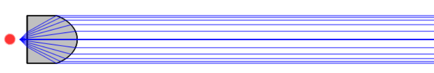
Figure 76: The effect of the Even Asphere lens on the source after optimisation of variables.
