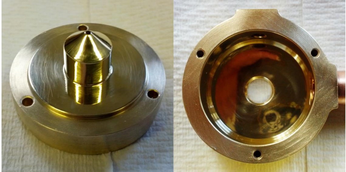
Figure 116: A picture of the upper (left) and lower (right) halves of the extraction head assembly after polishing.
