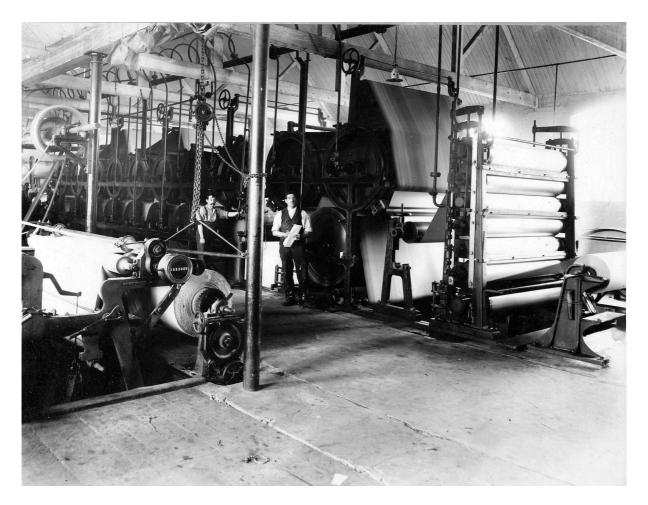
Fig 3: View of No. 2 machine's dry-end. On the far right the reel onto which the paper is rolled for further processing; before the reel one can see the calender stack. It is used to make paper surface smooth and glossy. In the background the series of steam heated drying cylinders (1907, Courtesy of Apsley Paper Trail).
