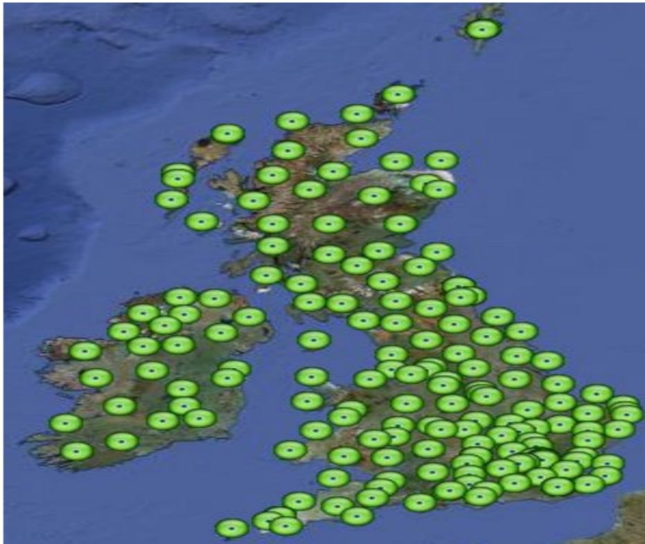
Figure 4.4: The BIGF ground-based GNSS network [image source: http://bigf.ac.uk/ ]
