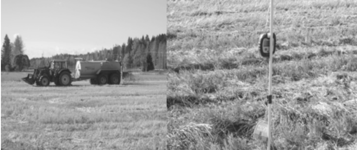
Figure 3. Both raw slurry and treated liquid fraction were spread by a broadcast spreader with a splash plate (left). Measurements were done with rugged temperature, RH and NH 3 sensors (right).
