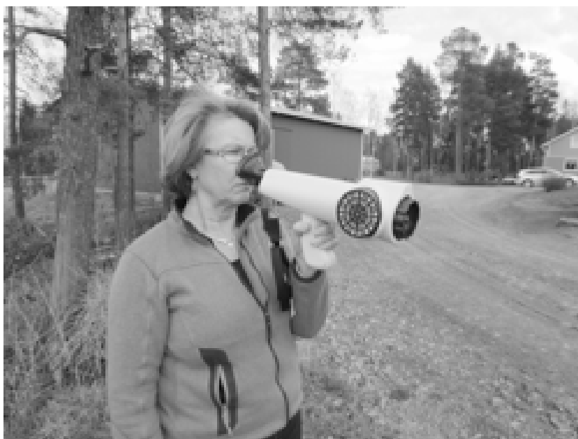
Figure 2. Odour measurements with Nasal Ranger™ field olfactometer
