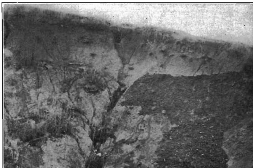
FIG. 48.—The Nebraskan gumbotil overlain by Kansan till in the road-cut between Sac and Crawford counties. Note how the Kansan stands with nearly vertical edge while the gumbotil surface has a decided slope.
