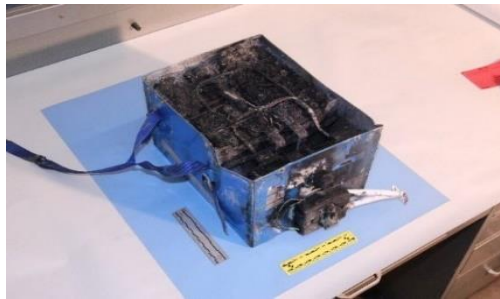
Figure 3 Catastrophe due to bad thermal management (Source: Wikipedia).
