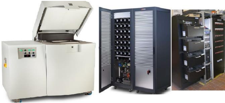
Figure 6 Experimental Framework Measurement Tools. [Left]Netzsch® Isothermal Calorimeter [middle]Digatron® Battery tester, [Right] Maccor® Battery Cycler.
