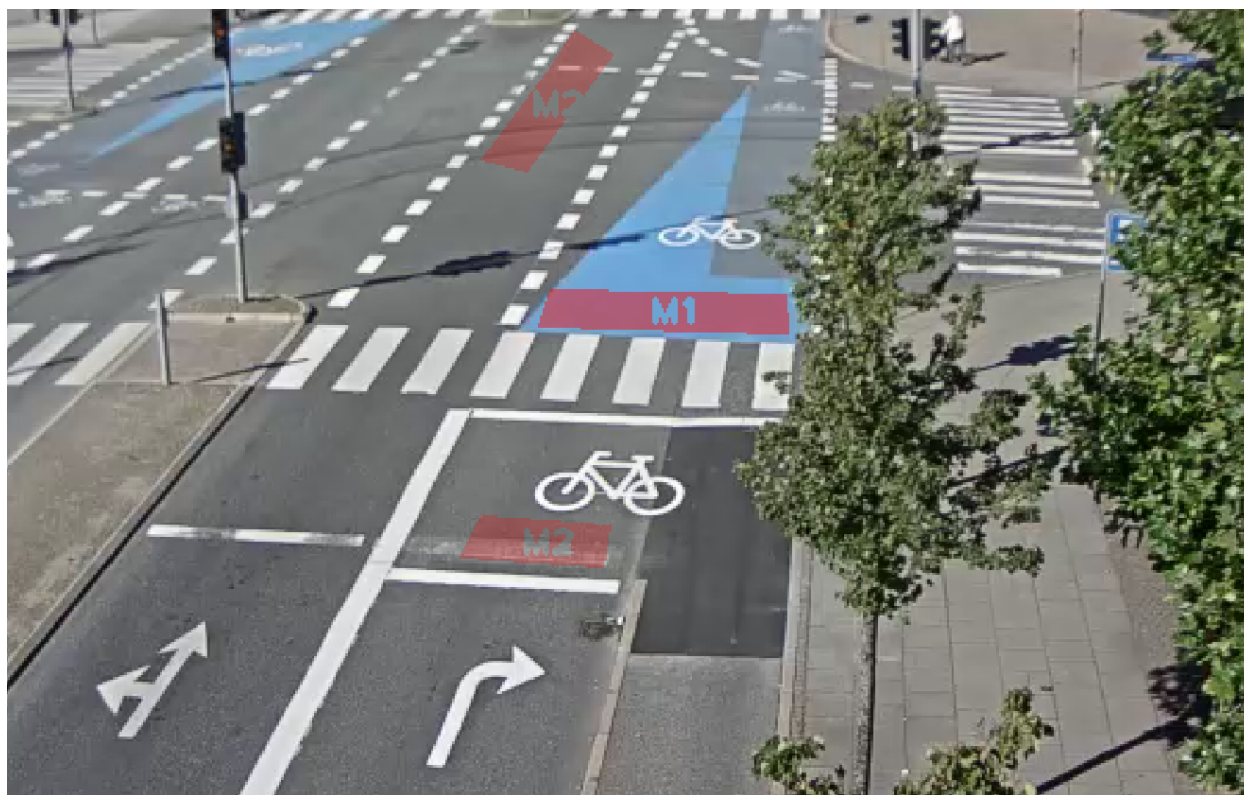
Figure 3: Double module to detect same time arrival between a straight going bicycle and a right turning car and a straight going bicycle and a left turning car.
