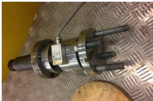
Figure 8.3. Head for hydraulic piston that is controlled by force
