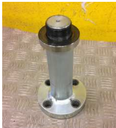
Figure 8.8. A 'displacement control' head for hydraulic piston
