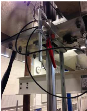
Figure 3.3. Displacement transducer clamped to the loading frame
