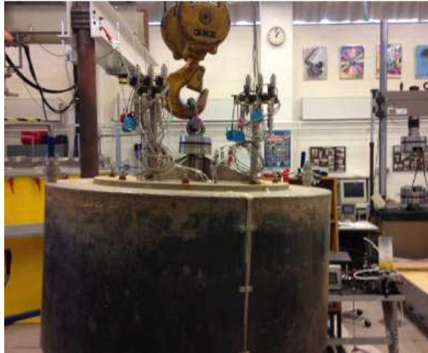
Figure 8.2. The bucket model lifted by crane
