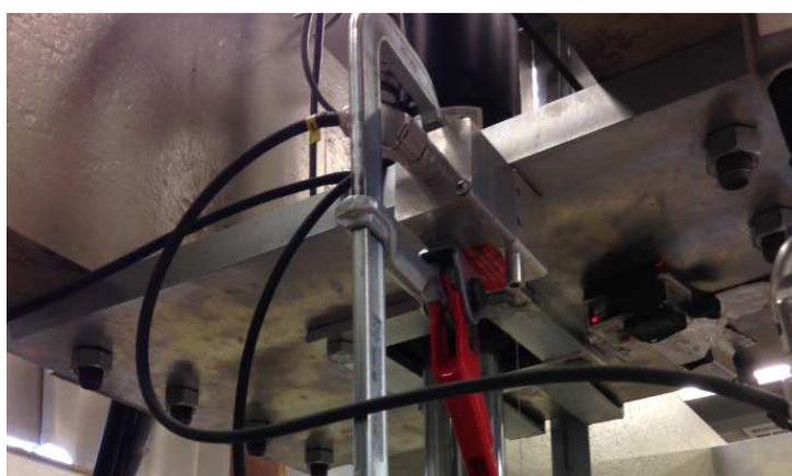
Figure 8.5. Displacement transducer clamped to the loading frame
