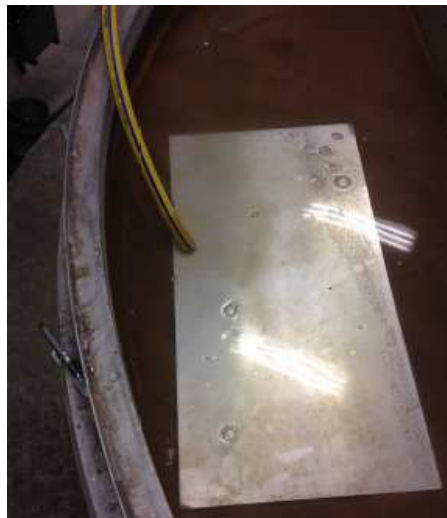
Figure 8.1. A plate and a hose used for raising the water level in sand box
