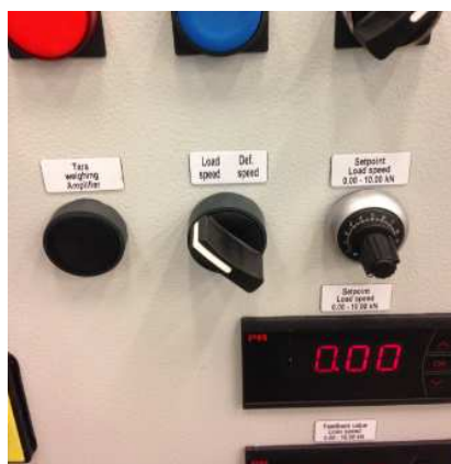
Figure 8.6. Control switchboard for the hydraulic motor: force set to 0.00.
