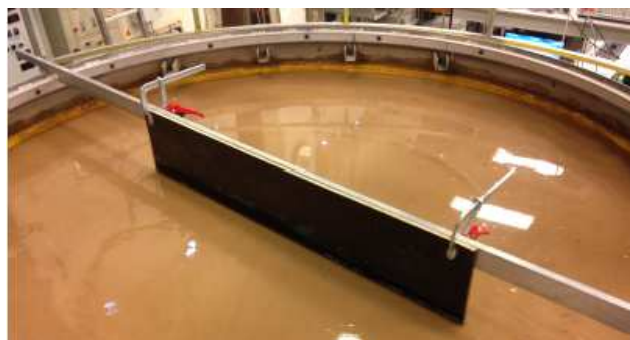
Figure 5.5. A beam with a wooden plate used for soil surface leveling
