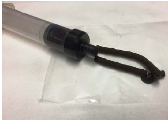
Fig 2 The syringe test applied to an alkaline pretreated feed showing the homogeneity of the feed after the test
