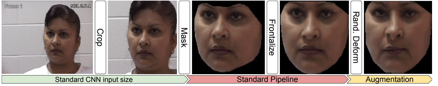
Figure 3: Pre-processing pipeline. The different stages of data pre-processing that were applied to the image. First, the image is aligned and cropped so as to fit the standard CNN input size. Then, it is masked and frontalized using piece-wise affine warping to match the standard pipeline proposed in [47]. Finally we perform data augmentation by applying landmark-based random deformations.
