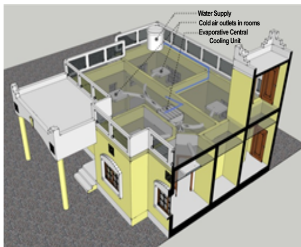
Figure 6: Illustration of the Evaporative cooling ducted air path system.
