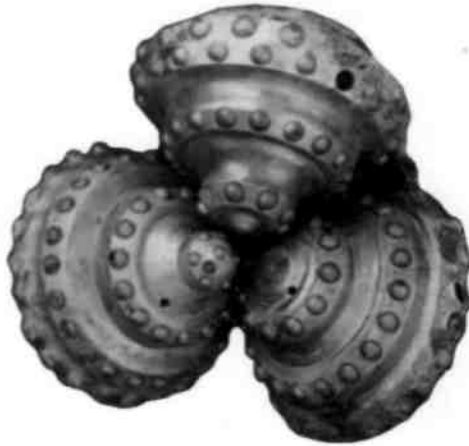
Fig.2 . Drilling bits 295 TK : fatigue destruction of collapsible hard-alloy teeth
