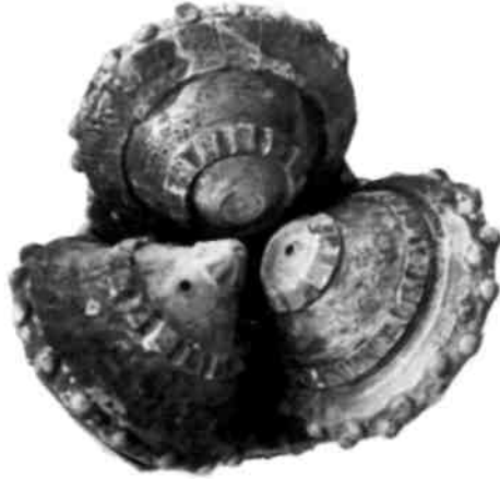
Fig . 1. Drilling bit 295 TK : abrasion wear of cutter tooth and fatigue destruction of plug pins
