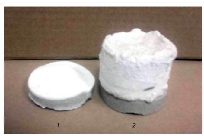
Figure 2. Filtration cake of clayless solution which is not weighted (1) and weighted by barite up to the density of 1820 \text{kg/m}^3 (2), after measuring at T = 140^\circ\text{C} and P = 5\text{ MPa}
