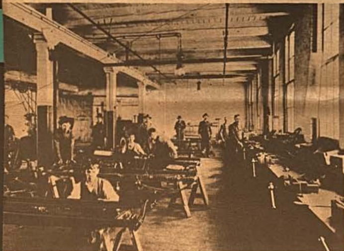
Up to the spring of 1913 the chassis for Model T's were assembled at fixed locations. Average assembly time per chassis was 14 hours.
