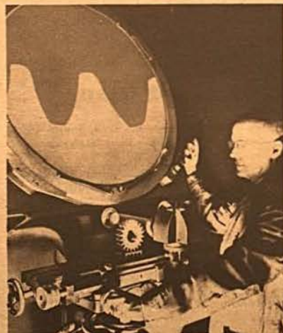
By magnifying a part or tool as much as 100 times, this comparator enables hairline checking of accuracy in machining.
