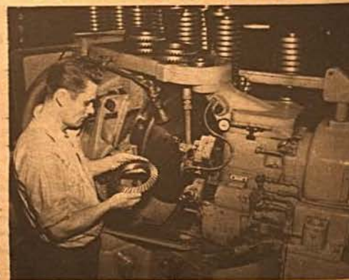
Crown gears for the rear axles of cars and trucks are cut on this high-precision machine of the very latest design.
