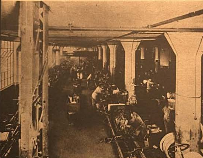
The moving assembly line reduced the time for assembly of a chassis from 14 hours to 1 hour 33 minutes within a matter of months.
