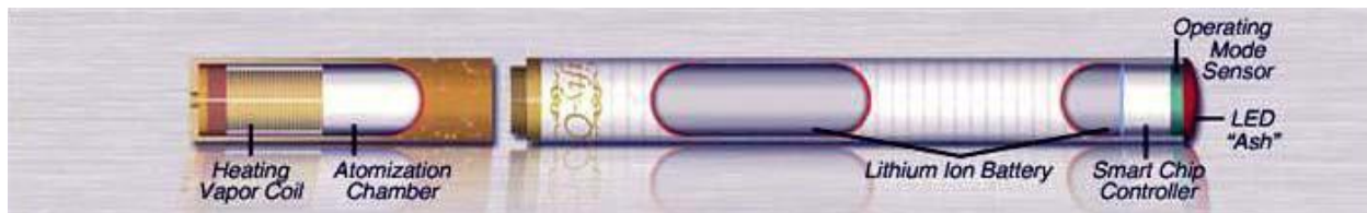
Figure 1. Electronic Cigarette Design (Wollscheid & Kremzner, 2009)
