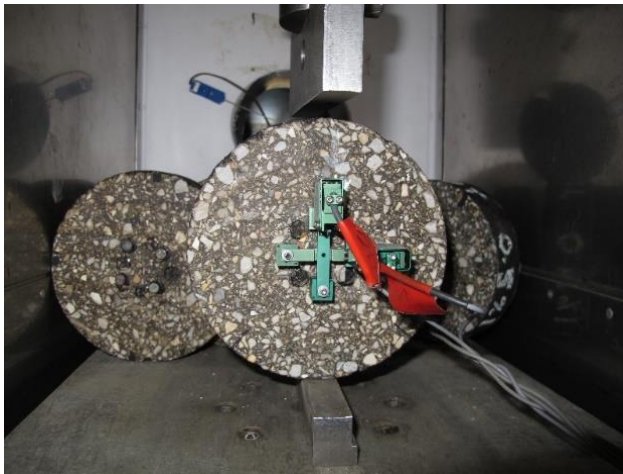
Figure 4.5 Dynamic Modulus in Indirect Tensile (IDT) Mode
