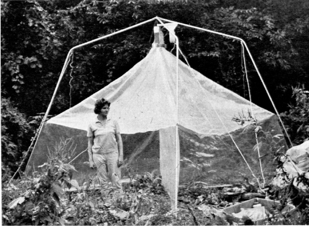
Figure 2. Large Malaise trap utilizing a prefabricated aluminum frame. After Marston (1965). Used with permission.
