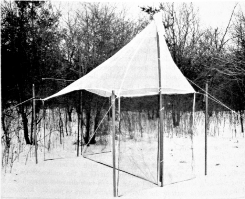
Figure 3. Townes' light-weight Malaise trap. After Townes (1972). Used with permission.
