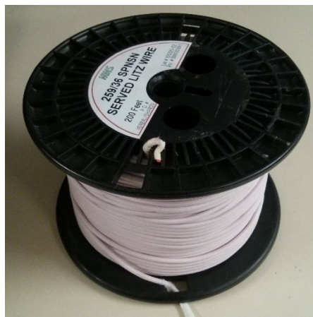
Fig. 4.4. Litz wire 259/36 for transformer prototypes
