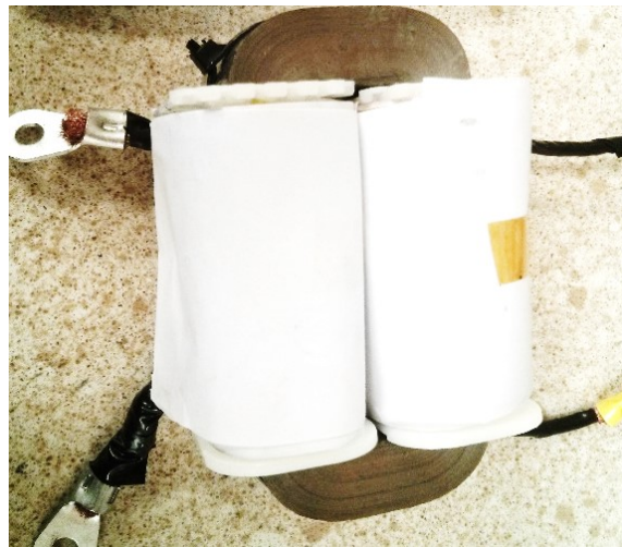
Fig. 4.6. Transformer prototype #2 in a core-type configuration
