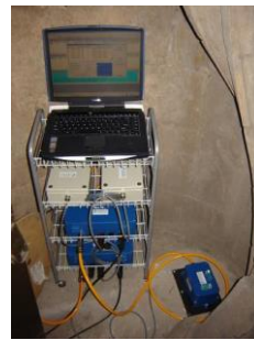
Figure 13 – Dynamic monitoring system [7]: (a) sensors location; (b) accelerometer A2 at the roof level; (c) battery of recorders and accelerometer A1 at the base level.
