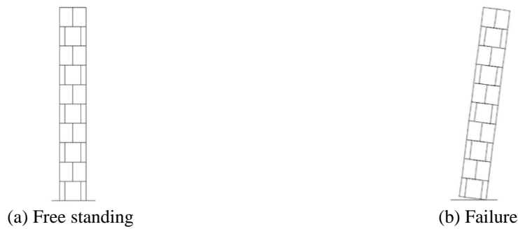
Fig. 6 (a) Stack bonded wall (b) collapse mechanism of stack bonded masonry wall under uniform pushover.
