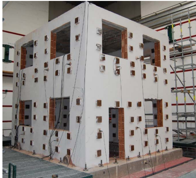
Fig. 3 Tested DLCW reinforced concrete structure (Leite, 2014)
