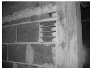
Figure 6 Crushing of loaded corner in a test specimen
