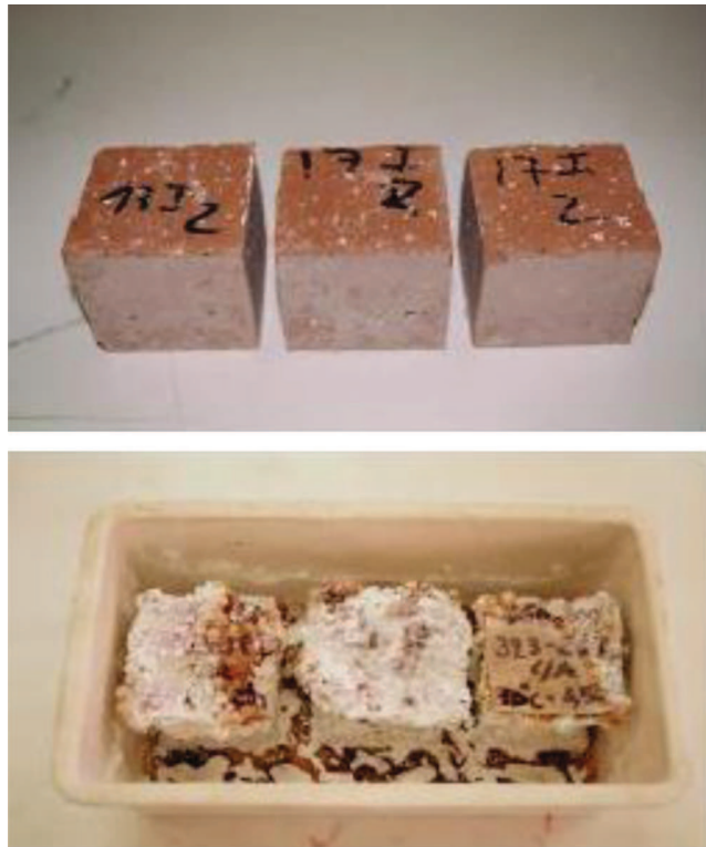
Figure 9.5 AACB mine-mortar specimens after water immersion. Above mortars based on plain mine-waste mud calcined at 950°C for 2 h. Below mortars based on mine-waste mud calcined at different temperatures with sodium carbonate. Reprinted from Pacheco Torgal F, Jalali S. Influence of sodium carbonate addition on the thermal reactivity of tungsten mine waste mud based binders. Constr Build Mater 2010;24:56–60. Copyright © 2010, with permission from Elsevier.
