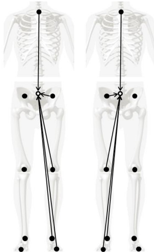
Figure 7 - Vectors for the Euclidean distances computed during the right gait cycle (right) and during the left gait cycle (left) for the LGGA calculation. The 3D components of each of these vectors are the input v in this index's equation.
