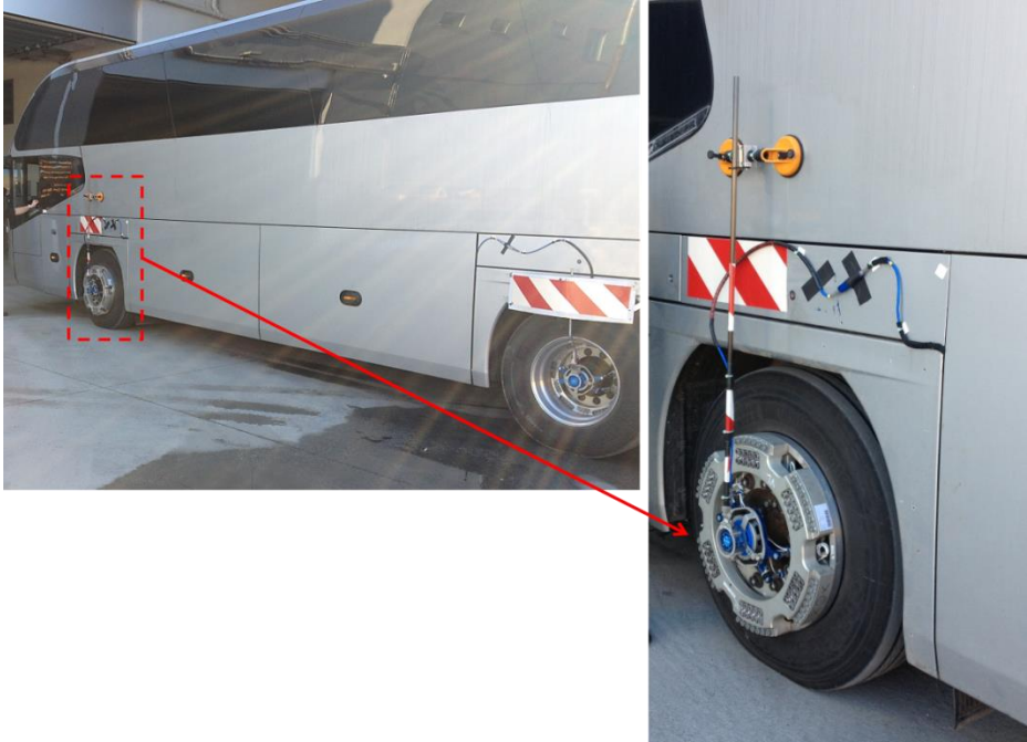
Figure 4.16 : Instrumented WFTs at the test vehicle.
