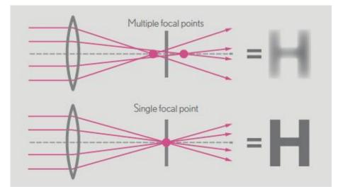
Figure 2.3: Spherical aberration (Url-4)
