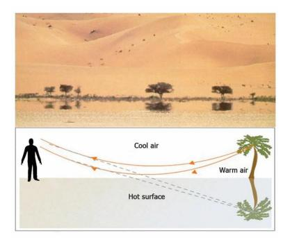
Figure 2.27: Sample of an Inferior Mirage and its scheme (Url-28)
