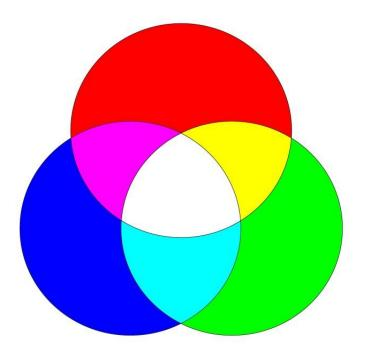
Figure 2.20: Additive color combination of RGB lights (Url-21)
