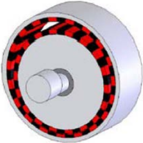
Figure 1.15: More practical harmonic magnetic gear [43].
