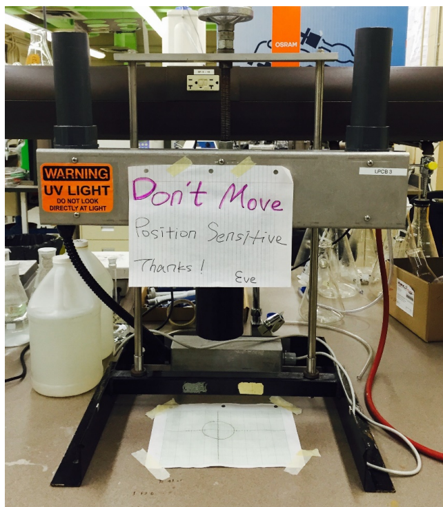
Figure A-3 UV bench-scale apparatus
