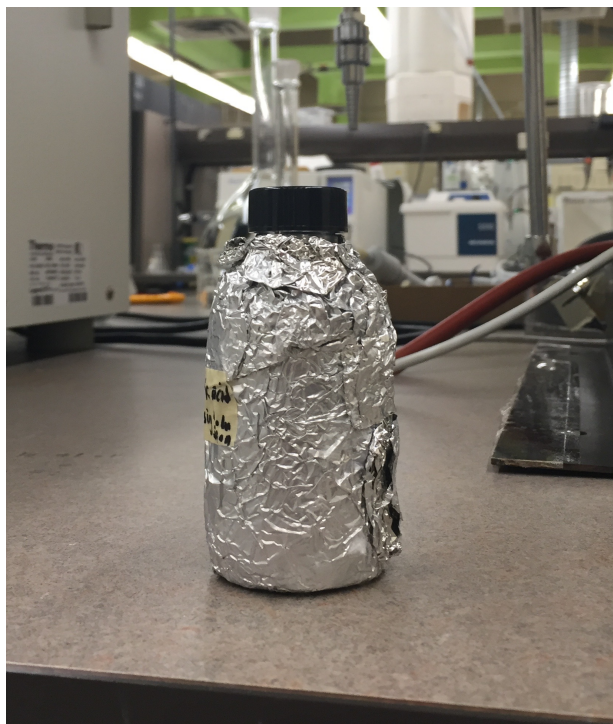
Figure A-7 Chlorination bottle with PTFE cap and aluminum foil
