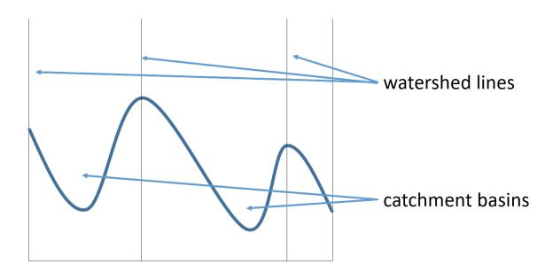
Figure 2.5: One-dimensional representation of watershed segmentation with a gray level profile of image data. Local minima yield catchment basins and local maxima define the watershed lines
