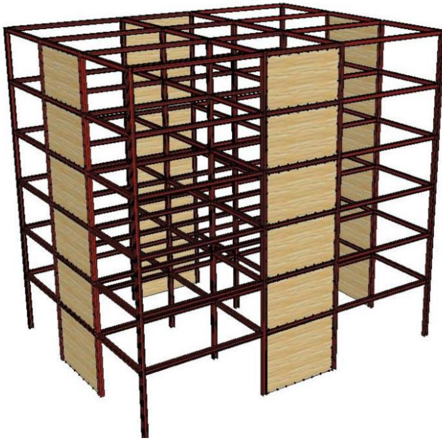
Figure 1: Steel-timber hybrid building: CLT infilled SMRFs
