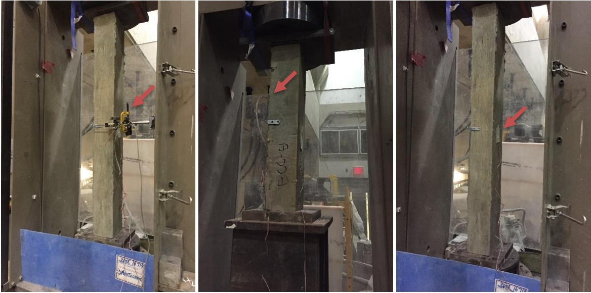
a) LVDT position b) Steel strain gauge c) Concrete strain gauge Figure 4: Column test setup and LVDT/strain gauges positions
