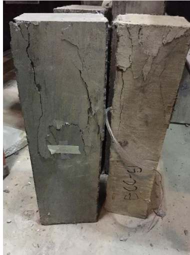
Figure 8: Crack patterns for ECC and UHPC columns under axial loading
