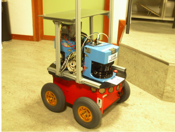
Figure 2.14: Pioneer 3-AT robot equipped with two laser range scanners.
