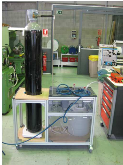
Figure 4.19: Petal \text{CO}_2 cooling system based on the open system developed by NIKHEF [94].
