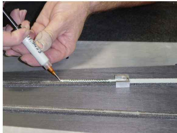
Figure 4.7: Tool used to control the height of the glue deposited on the POCO foam in the process of gluing to the carbon facing.
