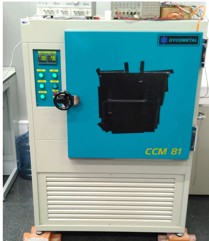
Figure 4.83: Climate chamber used for annealing procedure. The temperature and the humidity can be selected.
