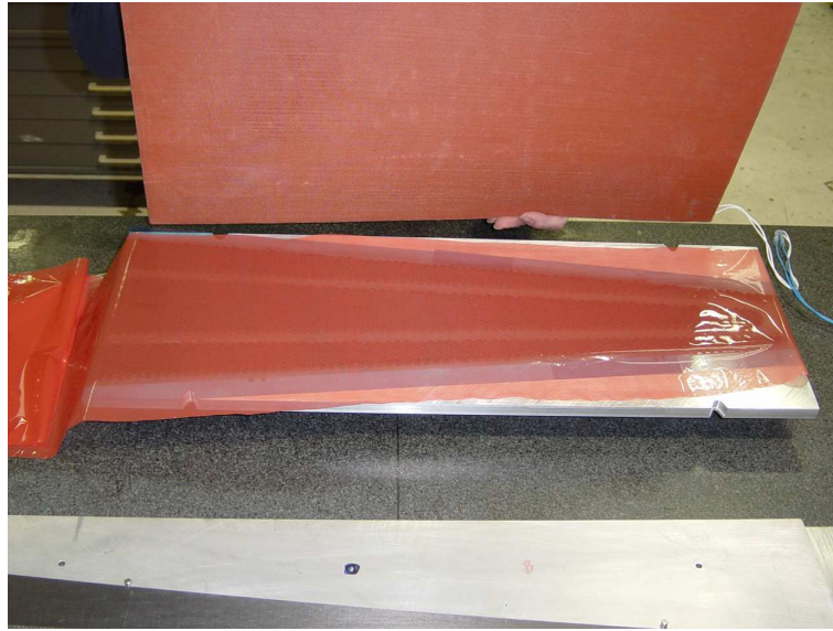
Figure 4.13: A thermal blanket is used to avoid any curvature in the honeycomb. A heat-resistant and anti-adhesive plastic is put between the honeycomb and the thermal blanket.
