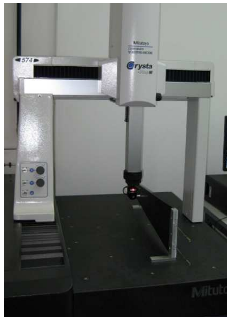
Figure 4.38: Coordinate measuring machine with a touch trigger probe where we measured the Petal in a “flag-like” configuration.
