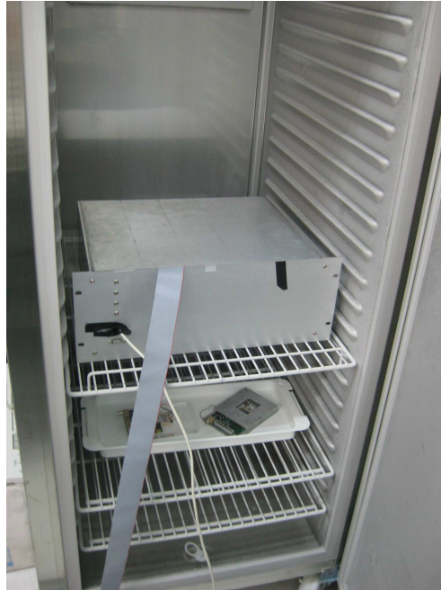
Figure 3.35: Charge collection measurement system placed inside a vertical freezer for measuring irradiated sensors. The temperature is maintained to -35^{\circ}\text{C} .
