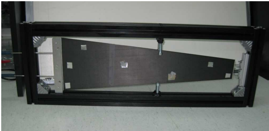
Figure 4.20: Metal support used to fix the Petal to the methacrylate box.
