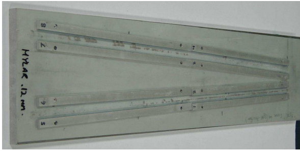
Figure 4.3: Aluminum platform used to glue the POCO foam and the pipes.
