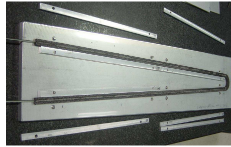
Figure 4.4: POCO foam and stainless steel pipes glued with CGL adhesive.
