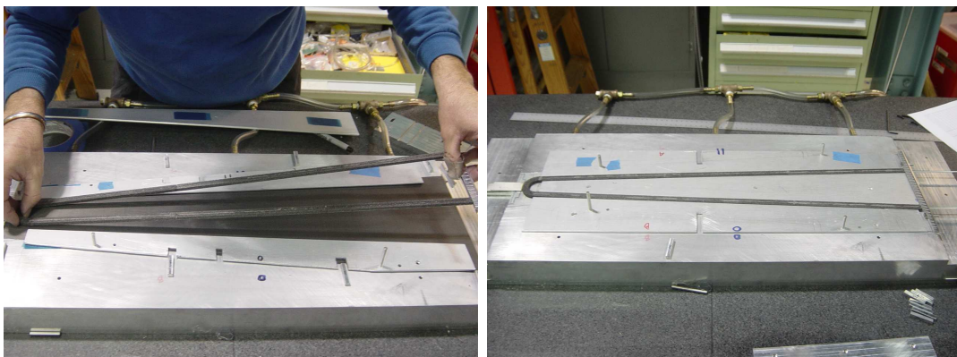
Figure 4.8: The foam is positioned on the facing using the aluminum sheets as guide (left) and then the central aluminum sheet is also placed (right).
