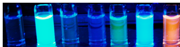
Figure 1. Samples contained Soman in MeCN mixed with each of the seven probes in DMSO. From left to right the samples contained probes BD00 to BD78.
