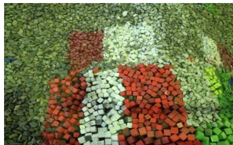
Figure 14 Fail in the 10 Tn blocks
