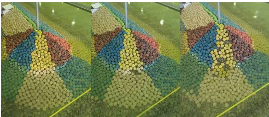
Figure 6. Evolution of damage ( I_{rp}=5.0, h=32 cm and R=52 cm) for H_s=8, 10 and 11 cm.
