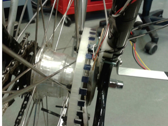
Figure 3.8: Rear wheel speed sensor with toothed crown and photoelectric sensor.
