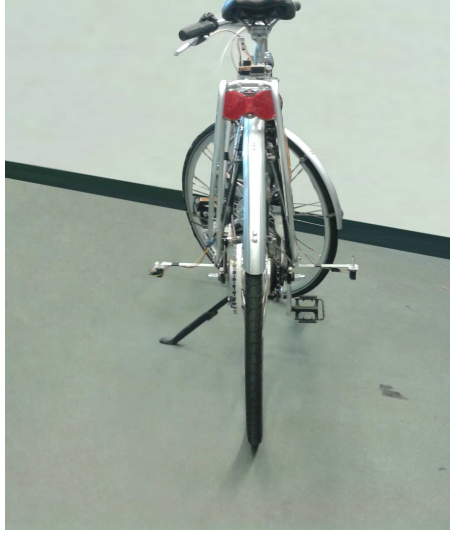
Figure 3.7: Bicycle rear view with left and right distance sensors for roll angle validation measurements.
