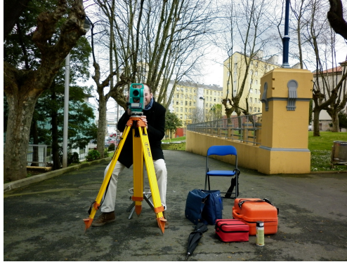
Figure 3.24: Topographical survey with the total station
