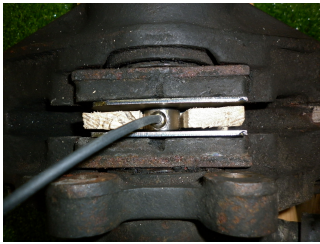
Figure 5.6: Load cell between the brake pads.
