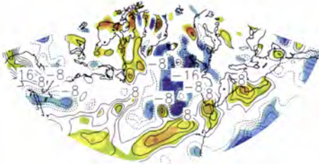
Figure 3.53: Difference of the vertically-averaged (500 – 300 hPa) mean horizontal divergence of humidity between dry and wet winters (contours) in 10^{-10} \text{ m.s}^{-2} and the corresponding p-values of the Student's t-test (shading) in the North Atlantic sector between 20^{\circ}\text{N} - 80^{\circ}\text{N} and 100^{\circ}\text{W} - 40^{\circ}\text{E} .
