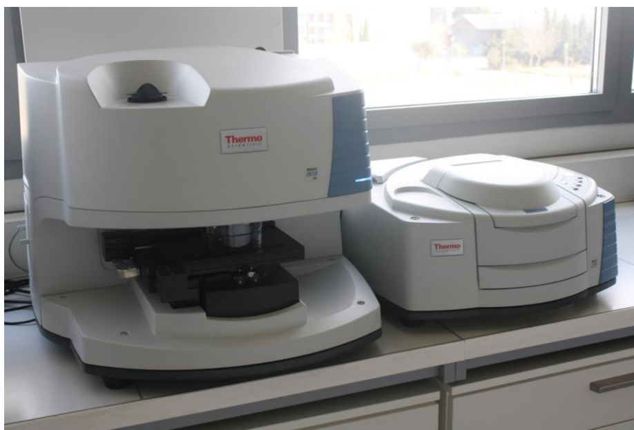
Fig. 24. Thermo Scientific™ Nicolet™ iS™10 FTIR Spectrometer (Source: Dauren Adilbekov, 2016)
