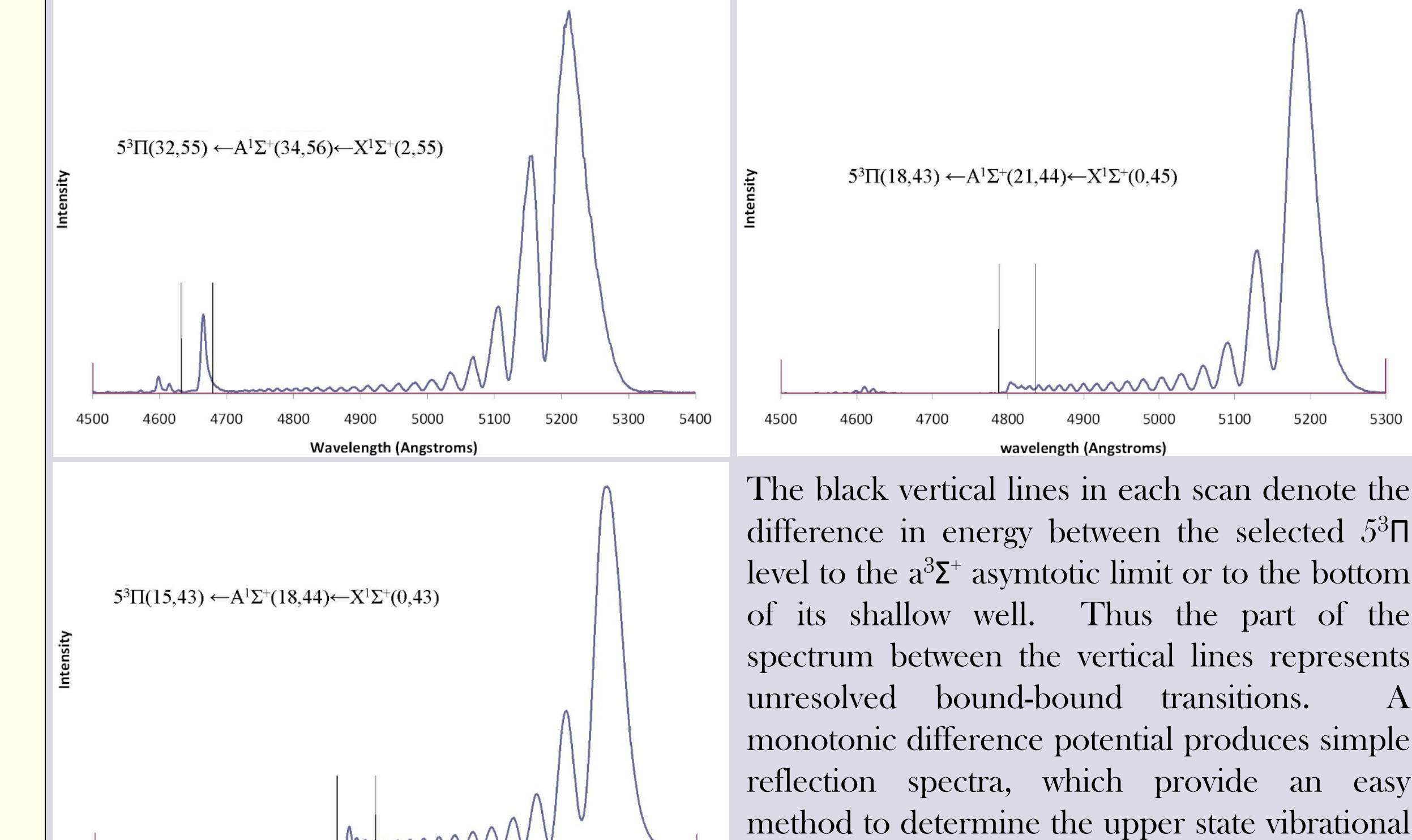
The black vertical lines in each scan denote the difference in energy between the selected  $5^3\Pi$  level to the  $a^3\Sigma^+$  asymptotic limit or to the bottom of its shallow well. Thus the part of the spectrum between the vertical lines represents unresolved bound-bound transitions. A monotonic difference potential produces simple reflection spectra, which provide an easy method to determine the upper state vibrational quantum number.
