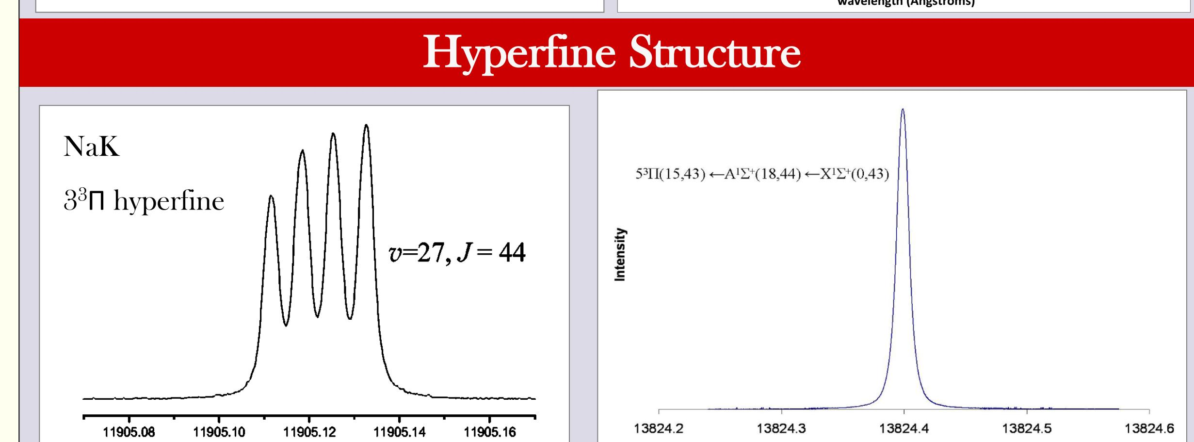
Previous work on NaK showed a rich variety of hyperfine structure. Ongoing studies of NaCs have yet to reveal clear hyperfine structure.
